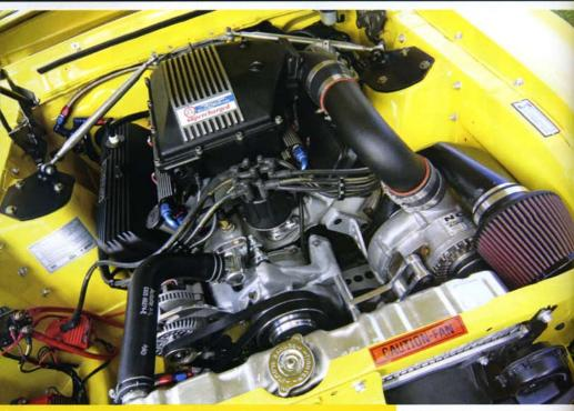
THIS COMBINATION OF GARGANTUAN FE DISPLACEMENT AND ABOUT 10 PSI OF CENTRIFUGAL BOOST MUSTERS NO LESS THAN 565 HORSEPOWER AND 558 LB-FT OF TORQUE AT THE REAR WHEELS, GIVING THE YELLOW JACKET A MUCH BIGGER STING THAN THE GREEN HORNET'S
