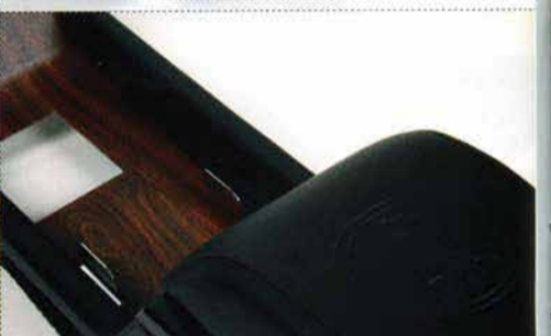
MPC sources the ashtrays from Shelby's original supplier—which, by the way, originally manufactured them for Cessna aircraft. These rear panels can be had with the light and ashtray combo, with the light alone, with the light and a power-point, or plain like the one in our lead photo.
