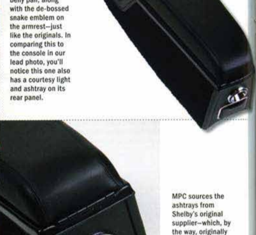
MPC sources the ashtrays from Shelby's original supplier—which, by the way, originally manufactured them for Cessna aircraft. These rear panels can be had with the light and ashtray combo, with the light alone, with the light and a power-point, or plain like the one in our lead photo.
