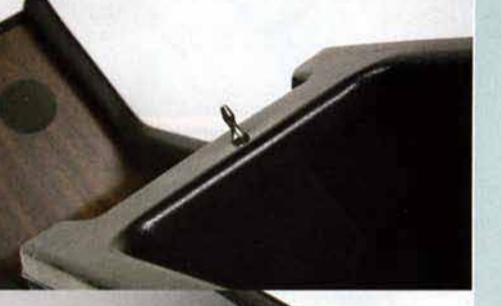
MPC's console storage bin is an ABS vacuum molding, and can be had in either its natural finish or lined with a felt flocking like the originals. The console's metal "belly pan" is shipped flat to MPC, pre-drilled and with or without laser-cut gauge and tranny-shifter openings. For utter consistency, the flat pans are then jig-formed at MPC to the proper shape. Depending on customer preference, these pans can be either vinyl-coated steel (like Shelby's originals), or brushed aluminum.
