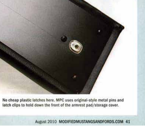
No cheap plastic latches here. MPC uses original-style metal pins and latch clips to hold down the front of the armrest pad/storage cover.
