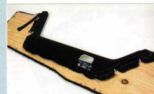
These extrusions are then skinned in vinyl (or leather) upholstery, making for soft, pliable edges on the console—much easier on the legs. The sides of the consoles are normally finished with carpet as shown here, but you can have them skinned in vinyl or leather, if preferred.
