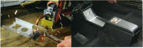
We mentioned that MPC's hinges come from Shelby's original supplier. Here, Peter is spot-welding one to a console's rear panel. Again, this is all done by hand, one at a time.
