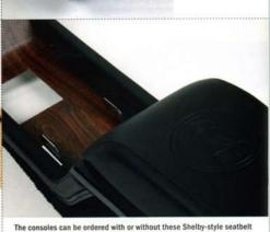
buckle clips. But note that these clips are dimensioned for Shelby buckles, which differed in dimensions from regular '68 Mustang buckles.
