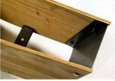
Just like Shelby's originals, MPC uses carriage bolts to secure the plywood walls to 18-gauge cross-braces and endplates. The result is a very rigid foundation that won't creak or squeak, like many a factory plastic console.
