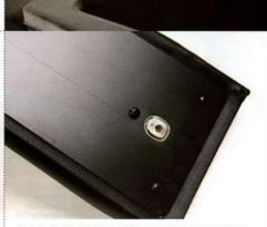
No cheap plastic latches here. MPC uses original-style metal pins and latch clips to hold down the front of the armrest pad/storage cover.
